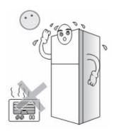
The unit should be placed on flat and steady ground. Keep the unit level by adjusting the front leg levellers.
